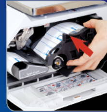
Cartridge loading type label installation
